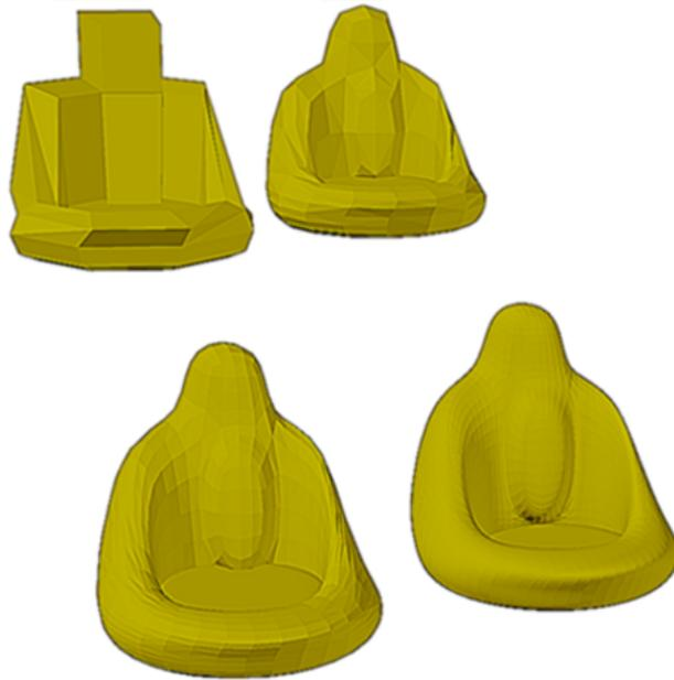
The lowest level of smoothness, or baseline, is 0. By default, Level 0 has no smoothness. You can increase the smoothness of any mesh object up to the current limits. However, you cannot decrease the smoothness of a mesh object whose level of smoothness is zero.
