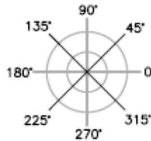
Absolute polar coordinates are measured from the UCS origin (0,0), which is the intersection of the *X* and *Y* axes. Use absolute polar coordinates when you know the precise distance and angle coordinates of the point.
