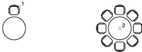
The radius of the array is determined by the distance from the specified center point to a *reference* or base point on the last selected object. You can use the default reference point (usually an arbitrary point that coincides with a snap point), or you can specify a new base point to be used as the reference point.
