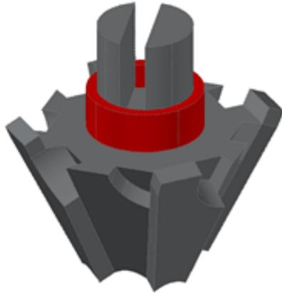
**object formed using press and pull operations on an imprinted pyramid**
