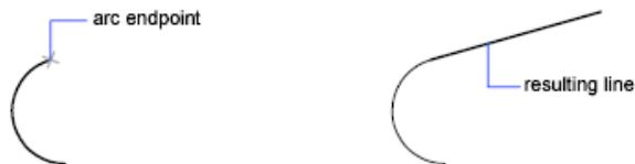
Immediately after you create a line or an arc, you can start an arc that is tangent at an endpoint by starting the ARC command and pressing ENTER at the Specify Start Point prompt. You need to specify only the endpoint of the new arc.
