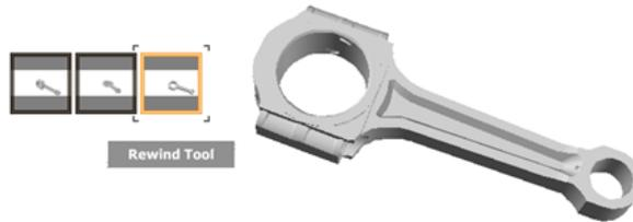
When a view change occurs, the previous view is recorded to the navigation history. If the view change is made with a wheel, a thumbnail is automatically generated and added to the Rewind UI. For view changes that are made not using a wheel, a thumbnail is only generated when the system variable *CAPTURETHUMBNAILS* is set to a value of 2. You can control when thumbnails are generated for view changes in the SteeringWheels Settings dialog box.
