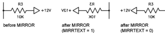
MIRRTEXT affects text that is created with the TEXT, ATTDEF, or MTEXT commands; attribute definitions; and variable attributes. Text and constant attributes that are part of an inserted block are reversed when the block is mirrored regardless of the MIRRTEXT setting.
