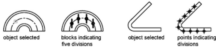
The starting point for measurements or divisions varies with the object type. For lines or open polylines, the starting point is the endpoint closest to the selection point. For closed polylines, it is the polyline start point. For circles, it is at the angle from the center point that is equivalent to the current snap angle. For example, if the snap angle is 0, the circle starts at the three o'clock position and continues counterclockwise.
