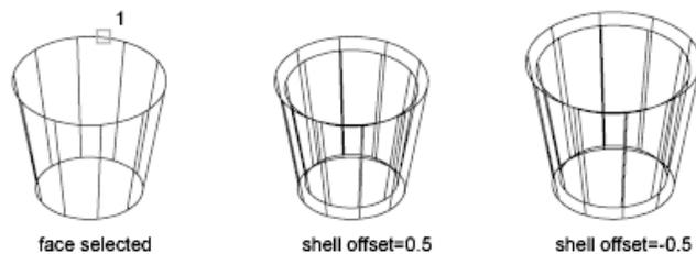
Continuously tangent faces are treated as a single face when they are offset.
