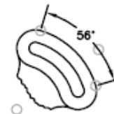
Two-Point Angular: extension line origins, and dimension line arc
