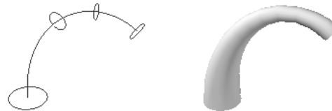
Cross sections with path curve
