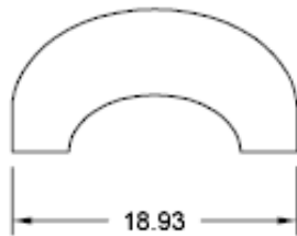
text centered vertically on the dimension line
