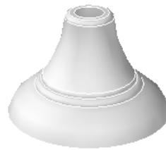
Revolved surface with modified profile
