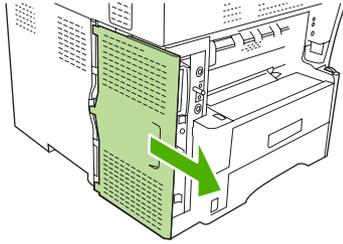
4. If necessary, remove the plastic fax-accessory cover from the formatter. Insert a coin into the groove at the top of the cover, and use it to pry the cover away from the formatter.
