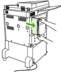
5. If you are replacing an existing fax accessory, pull up to remove it.
