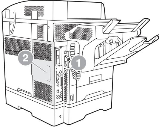
6. Open the formatter cage door (1) by pulling out on the door tab (2) and swing (3) the door open.
