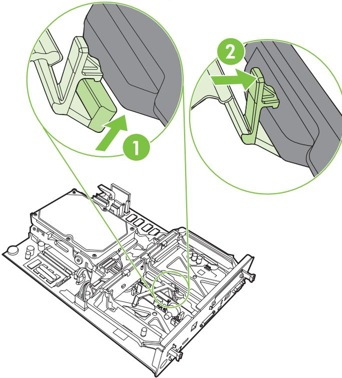
12. Secure the tab on the left side of the fax card strap.
