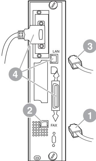
10. Connect the other end of the phone cord into the phone jack on the wall. Push the connector until you hear a click or until the connector is securely seated. Because there are different types of connectors, depending on the country/region, the connector might make an audible click when connected or might not make an audible click.
