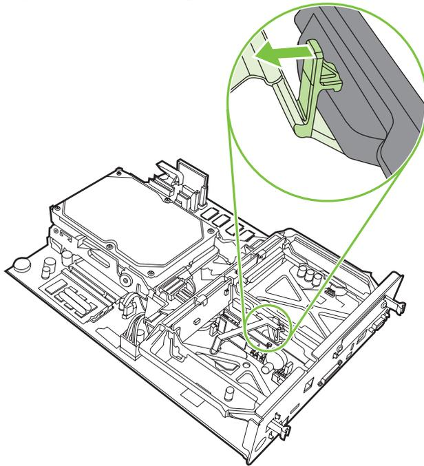
6. Lift up to remove the fax card strap.
