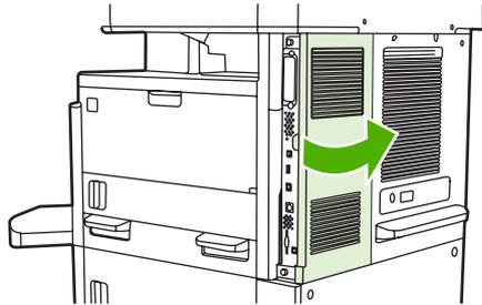
6. If you are replacing an existing fax accessory, unplug the fax cable and remove the accessory from the device.
