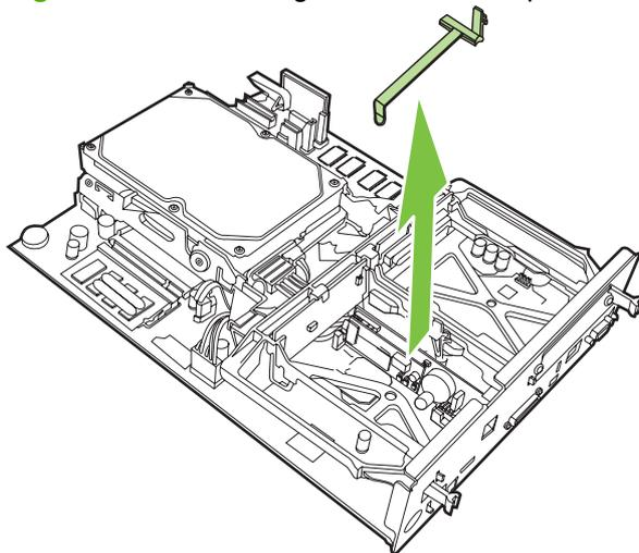
7. If you are replacing an existing fax accessory, pull up to remove it.
