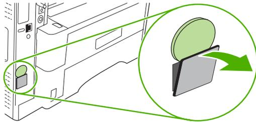
5. Open the formatter-cage door by grasping the metal tab and pulling the door open.
