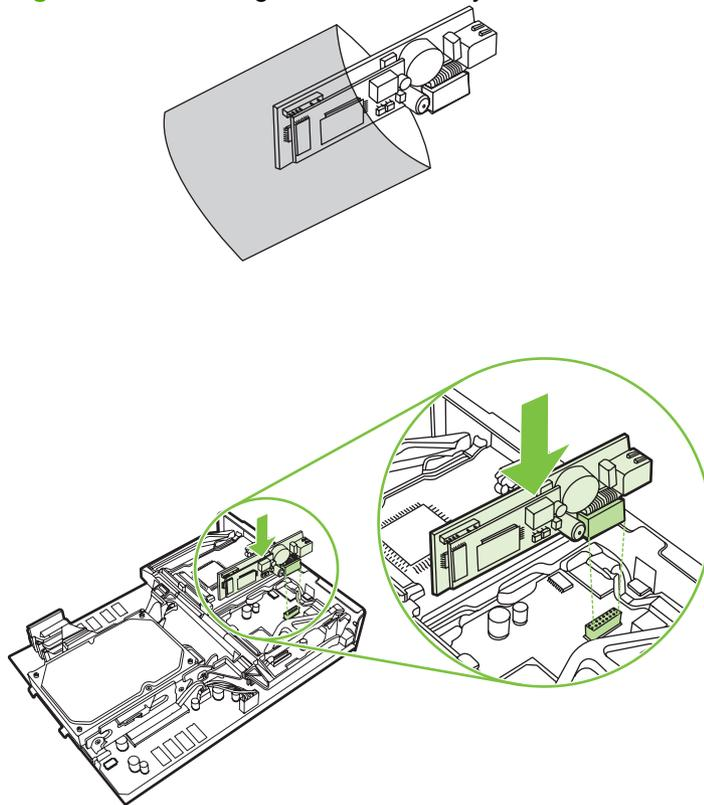
8. Slide the formatter board back into the MFP and tighten the two screws.
