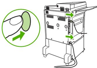
3. Loosen the two captive thumb screws on the back of the MFP.
