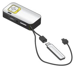
I Connect the USB storage medium to the USB socket of the cable
